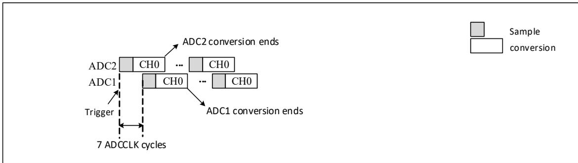
Note: The sampling time should be less than 7 ADC clock cycles, to avoid the overlap between ADC1 and ADC2 sampling phases in the event that they convert the same channel.
