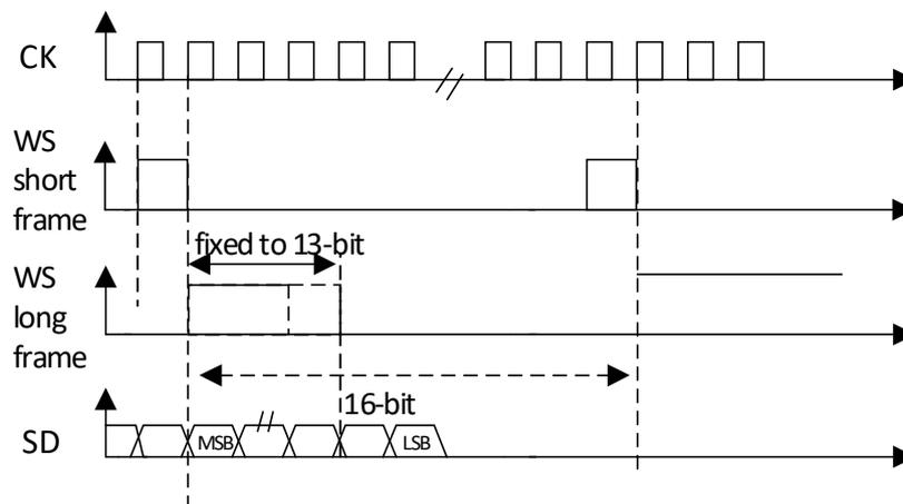
No matter which mode (Master or slave), which synchronization method (Short frame or long frame), the time difference between 2 consecutive frames of data and between 2 synchronization signals, (Even in slave mode) needs to be set by setting the I2SCFGR register determined by the DATLEN bit and the CHLEN bit.
