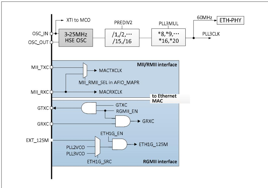
As can be seen from the above figure, the clock of the internal 10M Ethernet physical layer is provided by PLL3 and must be 60MHz. When using the internal physical layer, the second bit of the extension register needs to be set. After setting, the settings related to MII/RMII/RGMII are invalid.
