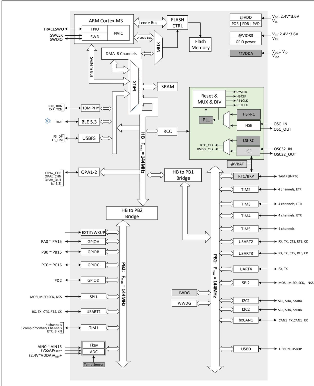
Figure 1-4 CH32V203 system architecture
