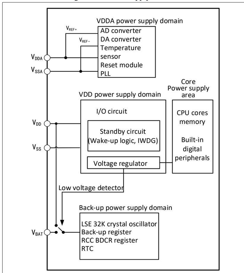
After the main power ( $V_{DD}$ ) is off, the analog switch will be turned to  $V_{BAT}$ , and the backup area will be powered by the  $V_{BAT}$  pin. At this time, the PC13 to PC15 IOs cannot be used as GPIOs, and only the following functions are available:
