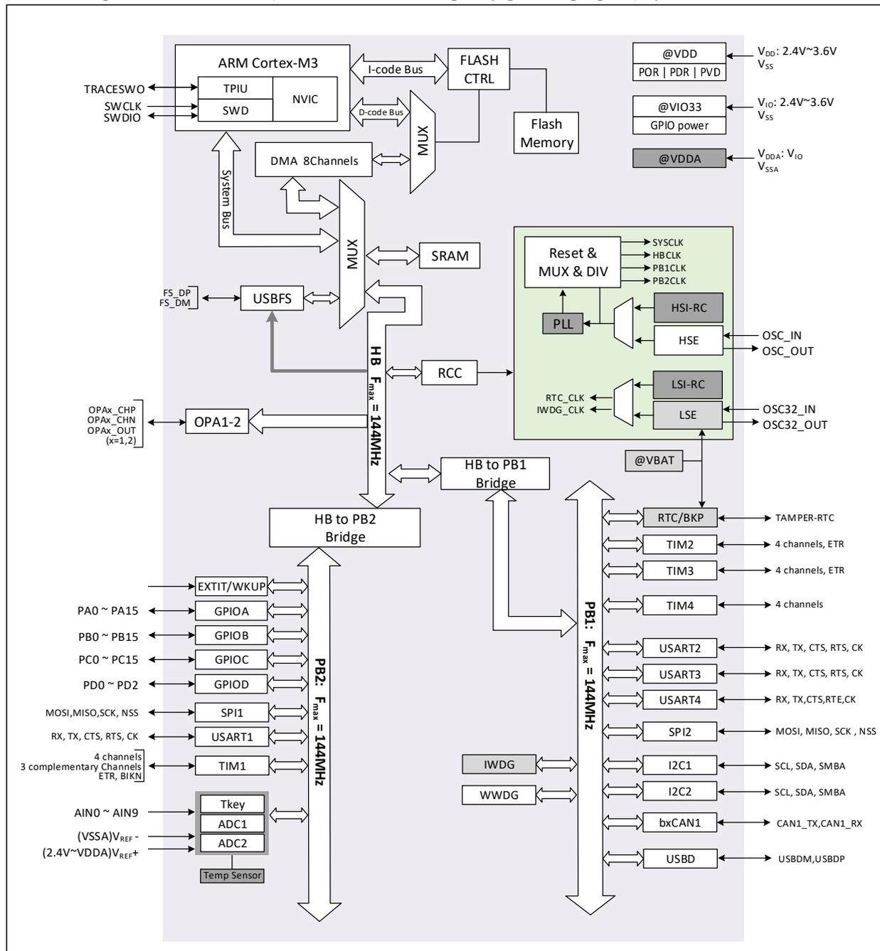
Figure 1-3 CH32F208 (Wireless) system architecture
