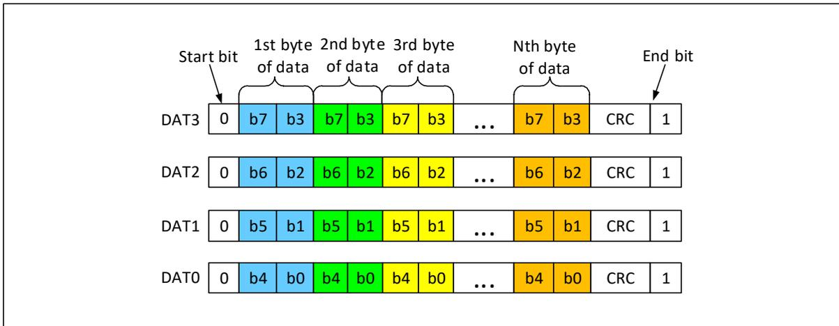
Figure 28-11 SD card single bus data transfer in a 512-bit word format
