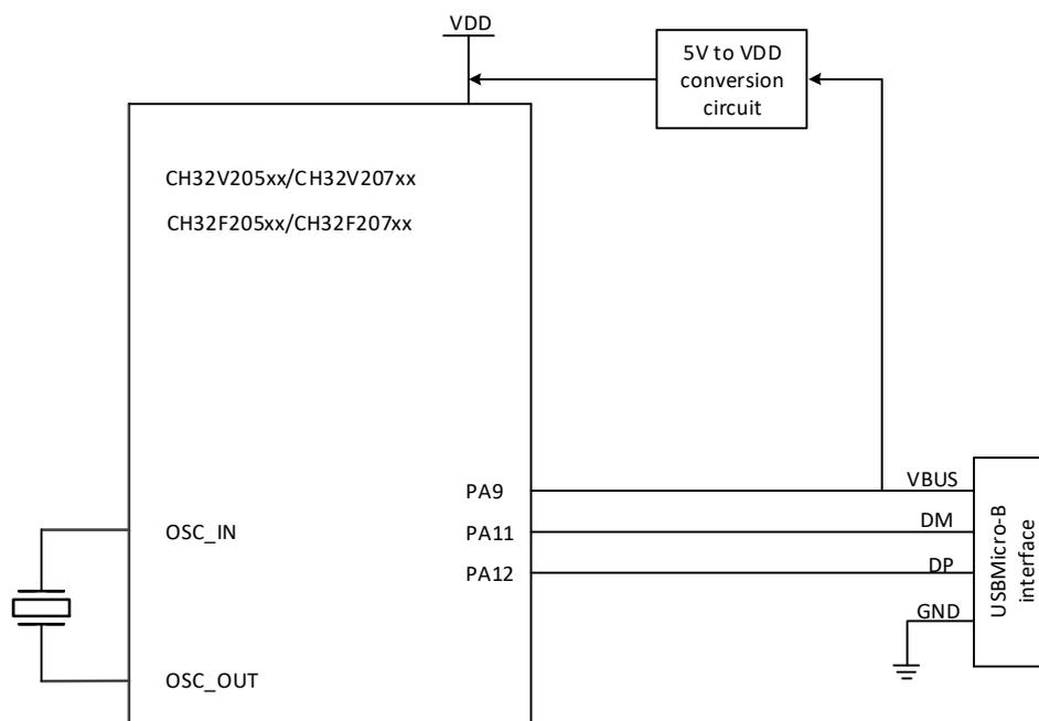
The USB bus pull-up resistor necessary as a USB device can be set by software at any time to enable or not. When RB\_UC\_DEV\_PU\_EN in the USB control register R8\_USB\_CTRL is set to 1, the controller is set according to the speed of RB\_UD\_LOW\_SPEED, which is the DP/DM pin of the USB bus internally. Connect a pull-up resistor and enable the USB device function.
