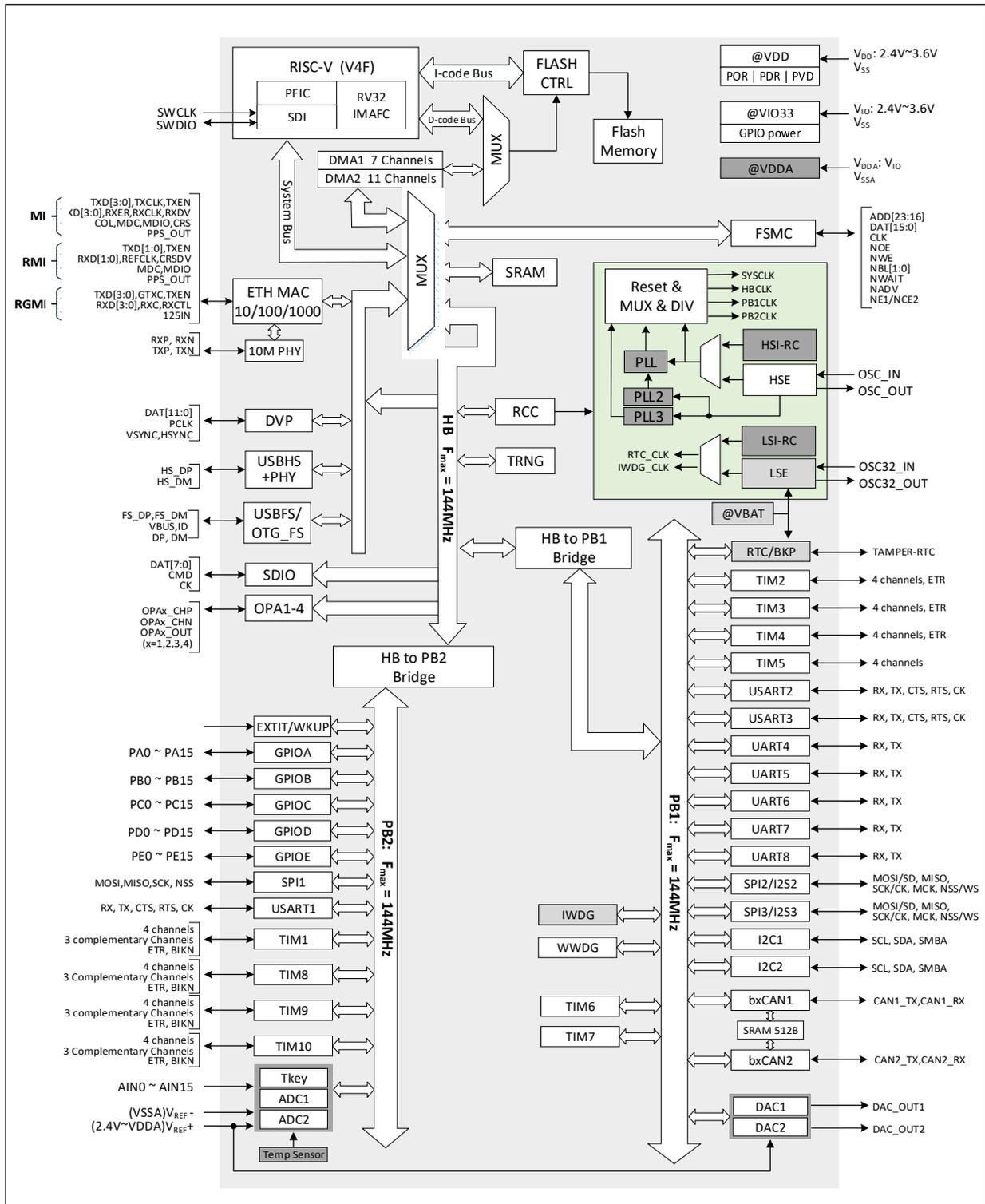
The system is equipped with: General DMA controller to reduce CPU burden and improve efficiency; clock tree hierarchical management to reduce the total operating power consumption of peripherals, while being also provided with actions such as data protection mechanism and clock security system protection mechanism to increase system stability.
