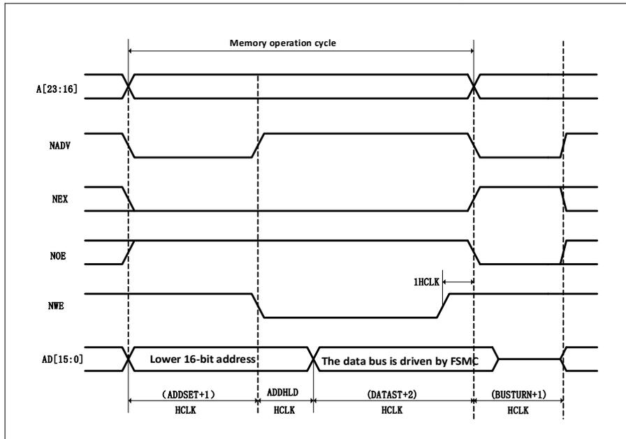
Figure 26-19 Mode D FSMC\_BCR1 bit field
