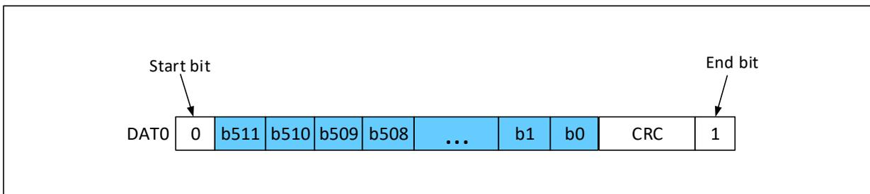
Figure 28-12 SD card 4 bus data transfer in a 512-bit word format
