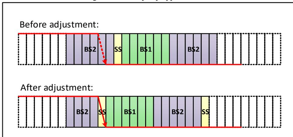
As shown in Figure 24-8, the SJW is 2, and the bus level transition is detected in the time period 2, so it is necessary to reduce the length of the time period 2 and reduce the SJW at the maximum, so as to advance the position of the sampling point.
