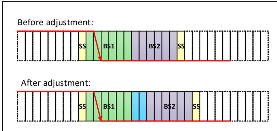
As shown in Figure 24-7, the SJW is 2, and the bus level transition is detected in the time period 1, then the length of the time period 1 needs to be extended, and the maximum SJW is extended, thereby delaying the position of the sampling point.
