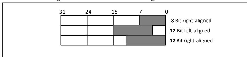
In dual DAC channel mode, there are also three methods: 8-bit data right alignment, 12-bit data left alignment, and 12-bit data right alignment.
