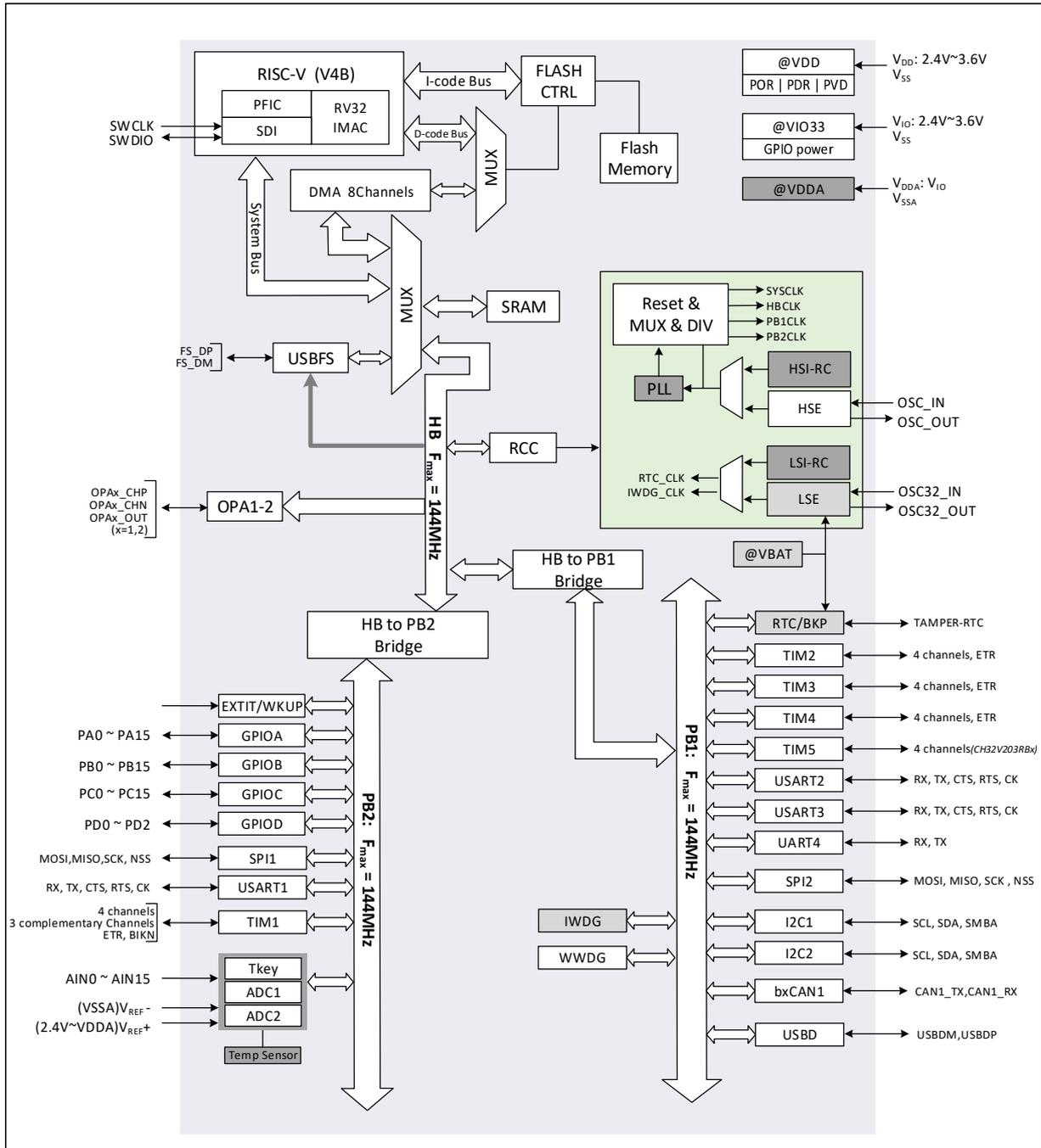
Figure 1-6 CH32V3x system architecture
