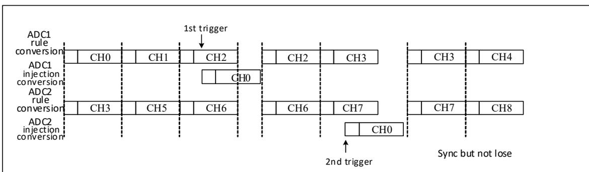
Note: In this mode, the conversion groups of ADC1 and ADC2 should have the same time, or the time of the longer conversion group is less than the trigger time interval.
