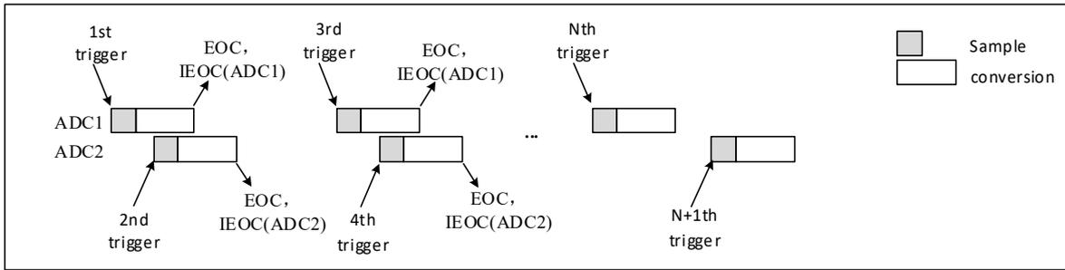
If the injected discontinuous mode is enabled, when the first trigger occurs, the first injected channel in ADC1 is converted. When the second trigger occurs, the first injected channel in ADC2 is converted. And so on. If an interrupt is enabled, an IEOC interrupt is generated after all injected group channels in ADC1 are converted. If an interrupt is enabled, an IEOC interrupt is generated after all injected group channels in ADC2 are converted.
