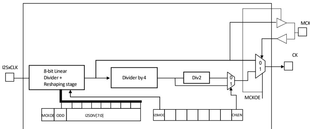
The clock source of I2SxCLK in the figure is the system clock (i.e., the HSI, HSE, or PLL that drives the HB clock). I2SxCLK can come from SYSCLK, or the PLL3 VCO (2xPLL3CLK) clock, which can be selected by the I2S2SRC and I2S3SRC bits in the RCC\_CFGR2 register. Audio can be sampled at 96KHz, 48KHz, 44.1KHz, 32KHz, 22.05KHz, 16KHz, 11.025KHz, or 8KHz (Or any value within this range). To obtain the desired frequency, set the linear divider according to the following formula:
