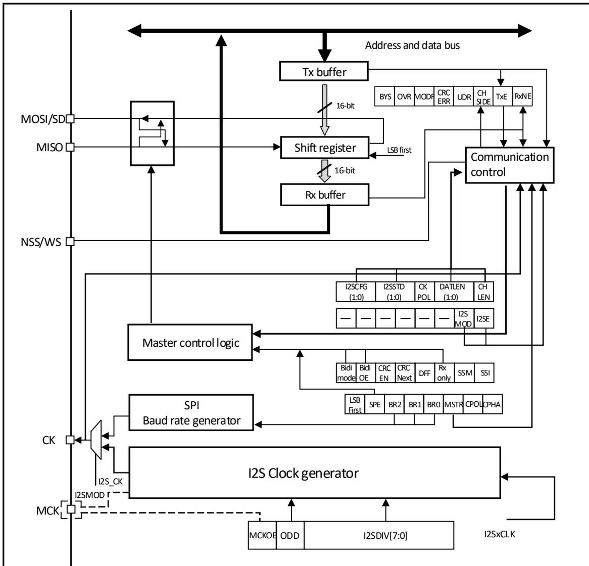
The I2S function is enabled by setting the I2SMOD bit in register I2SCFGR. At this point, the SPI module can be used as an I2S audio interface. I2S and SPI share 3 pins:
