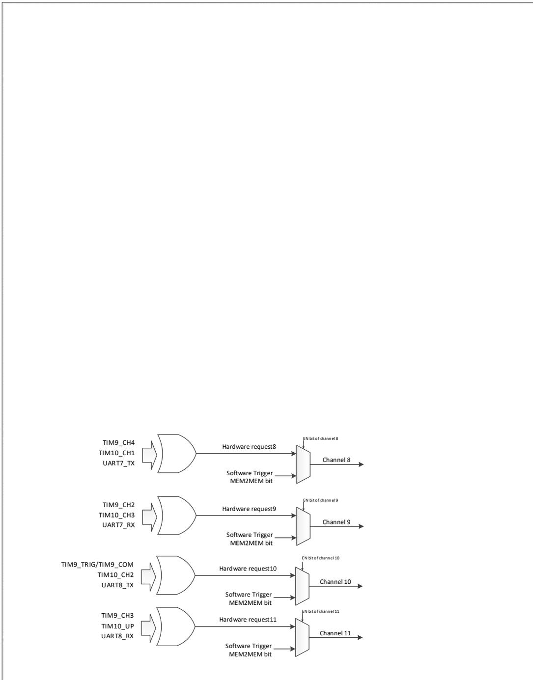
Table 11-2 Peripheral mapping table of each DMA1 channel
