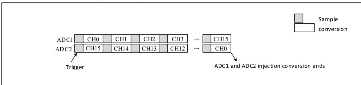
Note: 1. Do not convert the same channel on ADC1 and ADC2;
