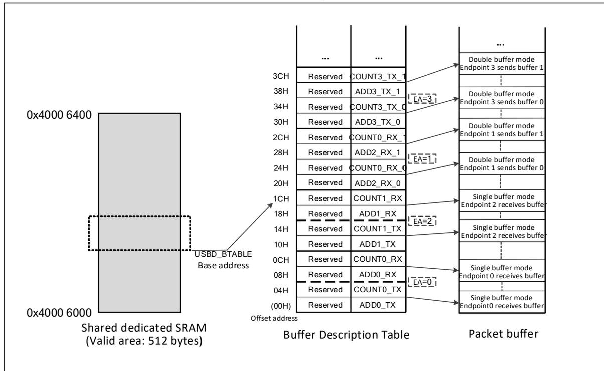
Whether receiving or sending, the packet buffer is used from the bottom. The USB module does not change the contents of other buffers beyond the currently allocated buffer area. If the buffer receives a data packet larger than itself, it will only receive data up to its own size, and the others will be discarded, that is, a so-called buffer overflow exception occurs.
