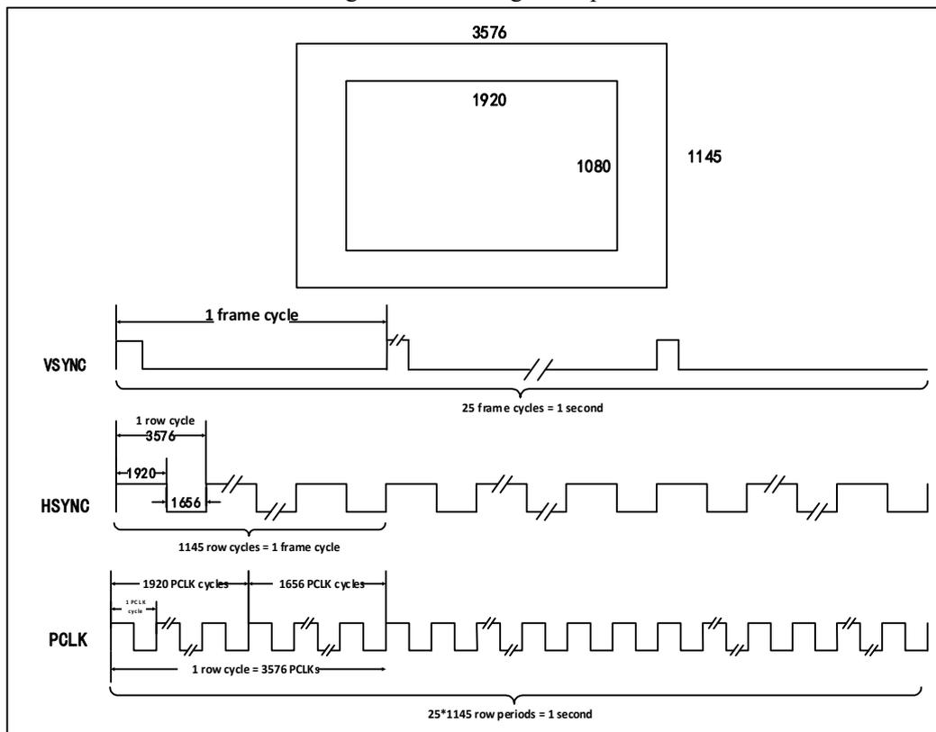
PCLK is the transmission time of a pixel, so HSYNC is 3576 times more than PCLK. Among the 3576 pixels, only 1920 pixels are valid, and the sensor does not transmit data during the remaining 1656 pixels. VSYNC is a frame synchronization signal, so the VSYNC time is 3576\*1145 times of PCLK. Similarly, the sensor is transmitting data only during the 1920\*1080 effective pixel time. If the sensor is transmitting JPEG compressed data, the HSYNC signal may not be needed.
