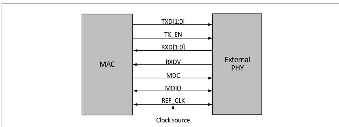
*Note: The Ethernet transceiver needs to input the externally provided REF\_CLK 50MHz clock frequency from the RXC pin.*
