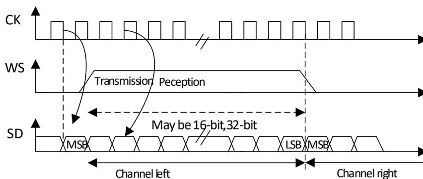
The sender changes data on the falling edge of the clock signal; the receiver reads data on the rising edge.
