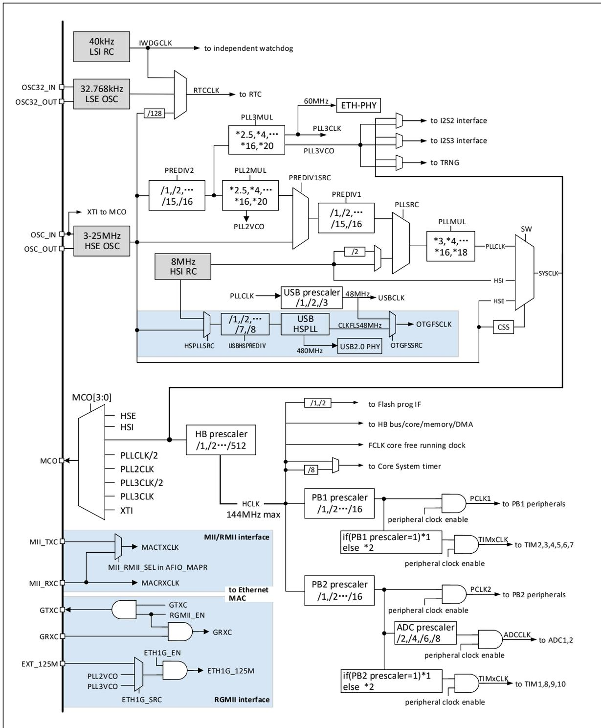
Note: This clock tree structure is applied for CH32F20x\_D8C and CH32V30x\_D8C.
