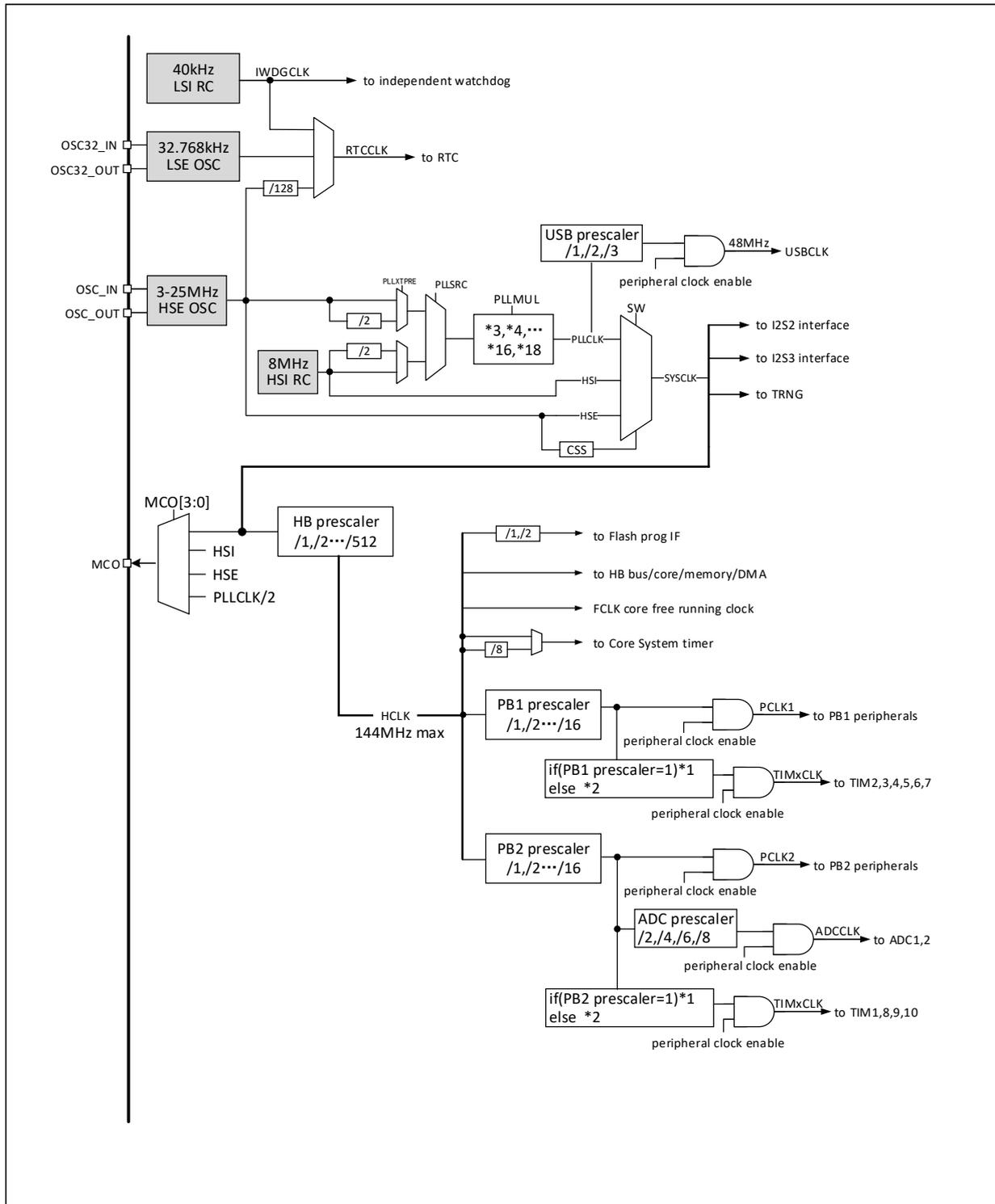
Note: This clock tree structure is applied for CH32F20x\_D6, CH32F20x\_D8, CH32V20x\_D6 and CH32V30x\_D8. When using the USB function, the CPU frequency must be 48MHz, 96MHz or 144MHz. when using the USB high speed function, the clock source of USBHSPLL can only be HSE. when the system wakes up from the stop or standby mode, the system will automatically switch to HSI as the main frequency.
