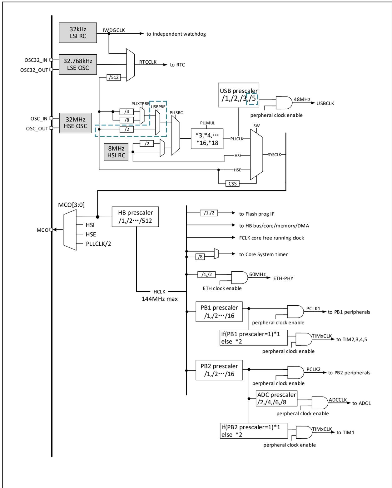
Note: (1) CH32V203RB (CH32V20x\_D8) products have an external crystal or clock (HSE) of 32M, and there is no need for a load capacitor to have been built in when using an external crystal.
